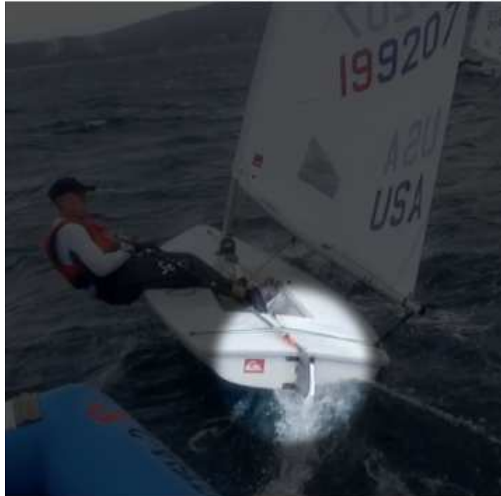
The tiller is up too much and the rudder drag is high. Too much weather helm.
