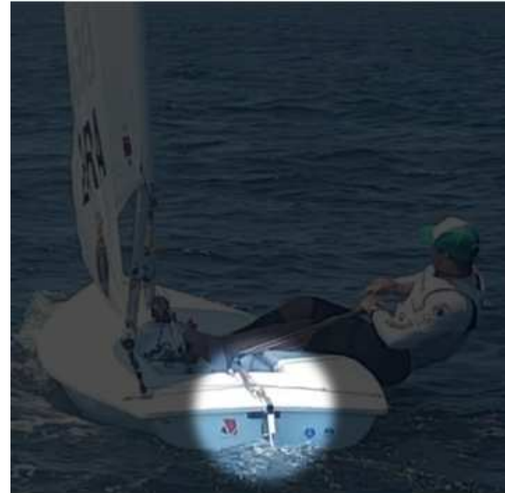
The tiller is just up a bit from centreline and the boat is balanced.
